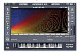
Take a sample as input and CUBE 2 analyzes it into two components: up to 512 sine tracks for the partial components and the residual spectrum for the noise components. The outstanding quality of the analyzer for a broad range of sounds avoids the typical artefacts known from time stretching/pitch shifting and granular algorithms.
